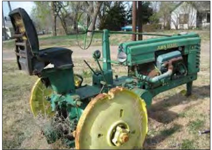
A John Deere B with a Corvette V-8 engine and an automobile seat.
