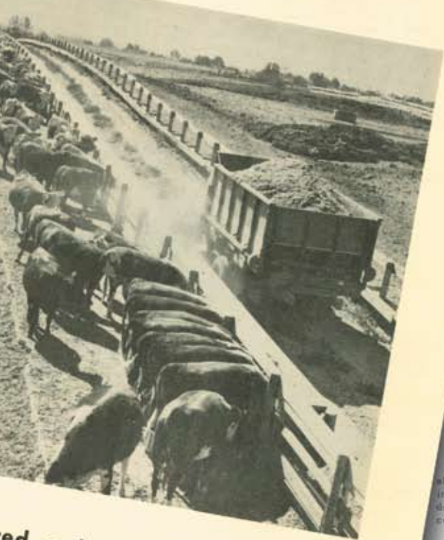
MECHANICAL FEEDING P. T. O. showing self-feeding mixer-unit.
